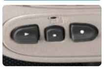
The Travel Note Recorder enables you to record a message and play it back later. The controls are located in the overhead console.
